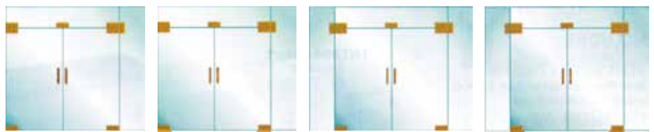
Paired doors, transom and sidelite with top and bottom manual pivots
